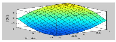
Figure 5. Surface viewer for cart controller
