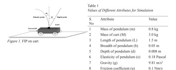
The equations for motion of the FIP system were derived as follows:
